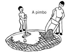
Figure 9: The mesh is covered with more concrete
