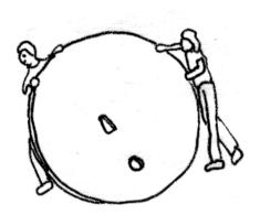
Trowel it flat. After it has set, splash water on the concrete and cover it with plastic sheeting. Keep it damp and covered with plastic for 7 days. After the concrete has cured for 7 days, roll the slab over to the latrine pit. Mortar the bricks and lay the slab on top.
